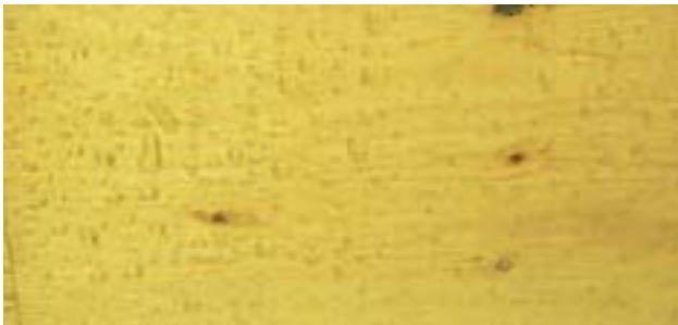
Photo shows example of the beading that occurs because of our coating process.
