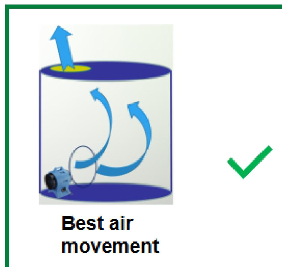
***Local Exhaust Ventilation (LEV) effective for localized generated air contaminants (i.e. welding, grinding, etc.)***
