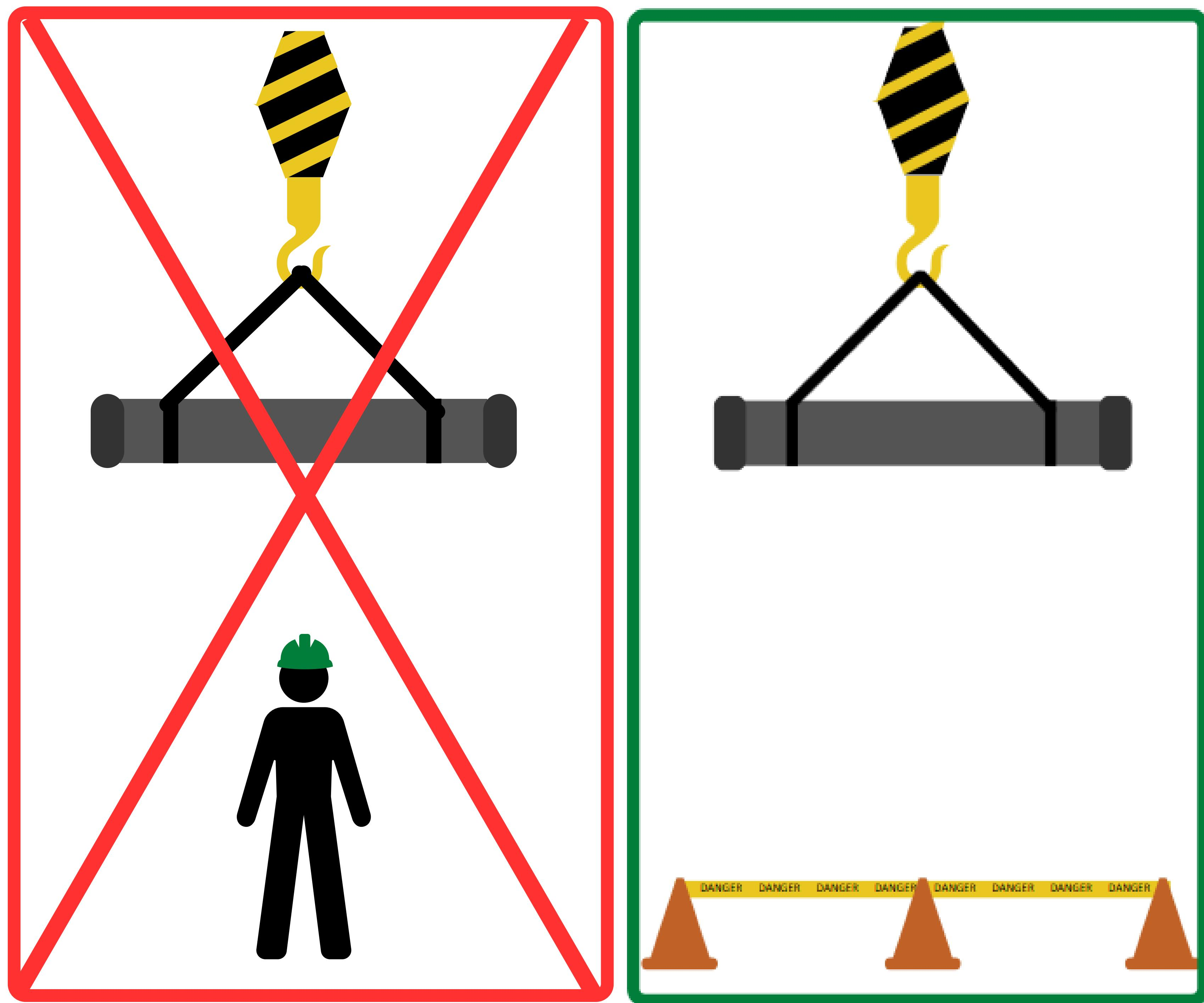
***Never raise a load higher than necessary, or leave a load suspended in the air. Clearly barricade the lifting zone before a lift is completed.***
