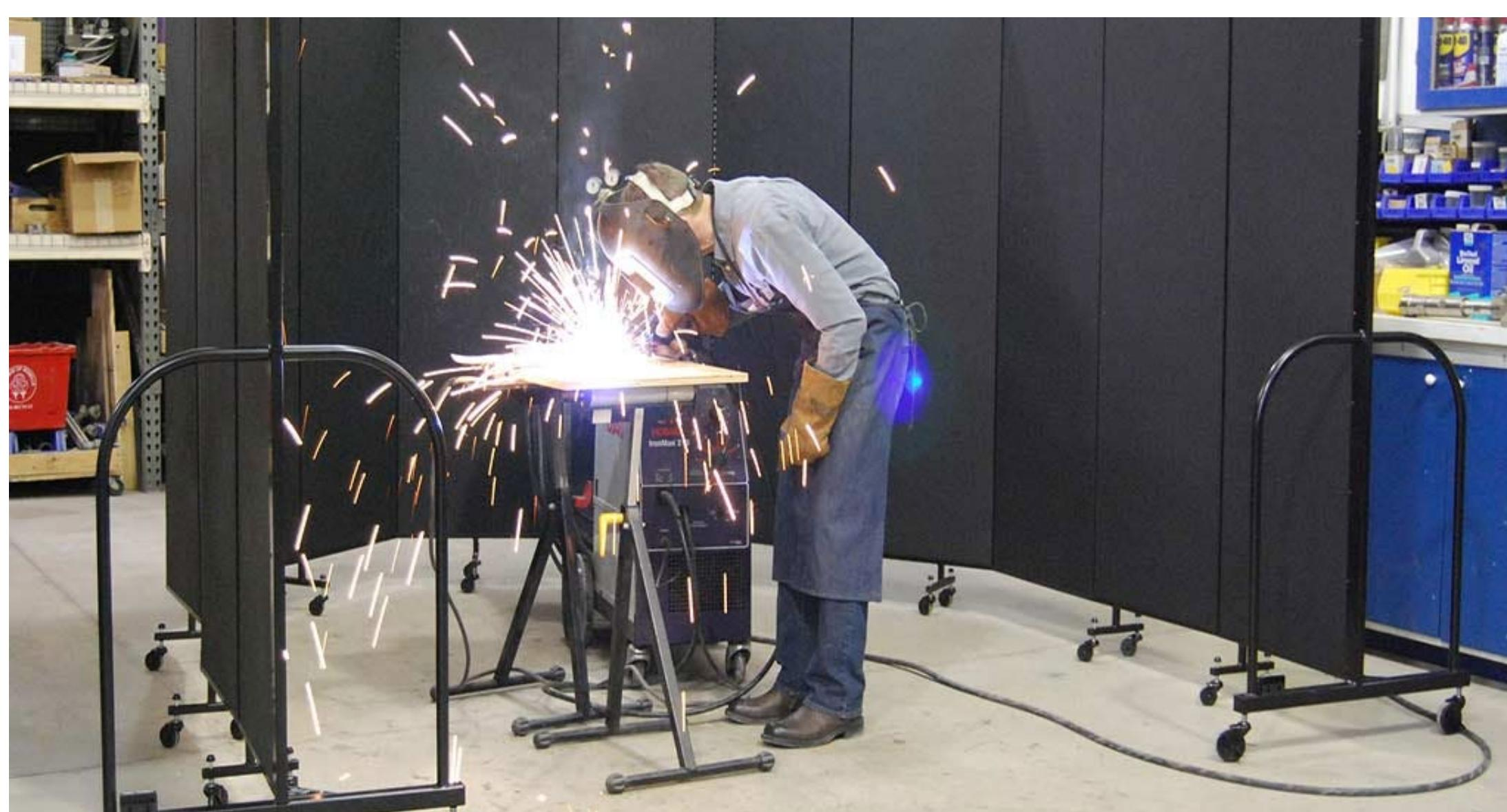
Many mills have had significant fires as a result of wind picking up hot embers, so areas exposed to drafts and wind must have a wind screen or some other barrier to prevent sparks from travelling far from the hot work area.
