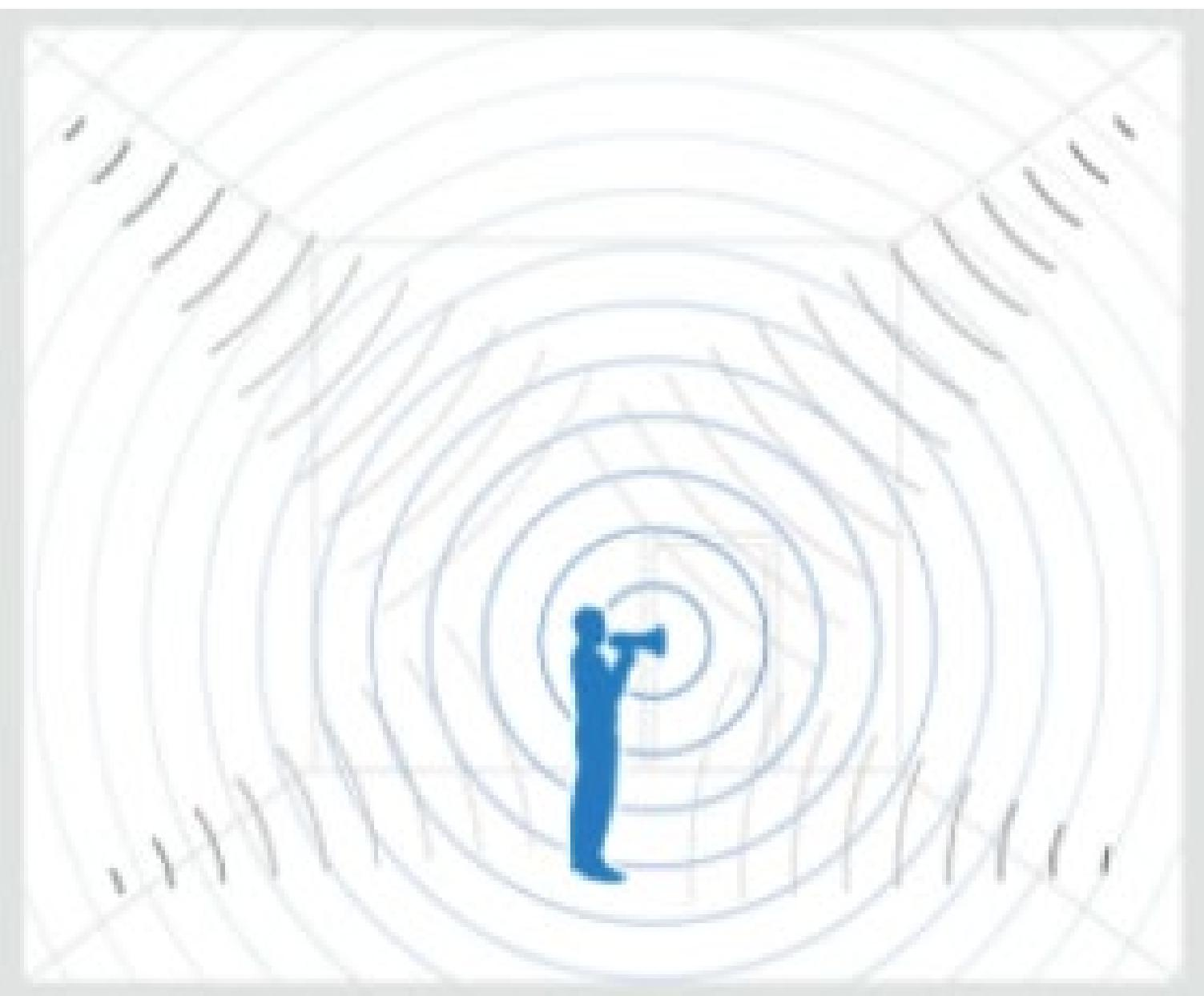
Noise levels from a source inside a small confined space can be up to 10 times greater than the same source placed outdoors!
