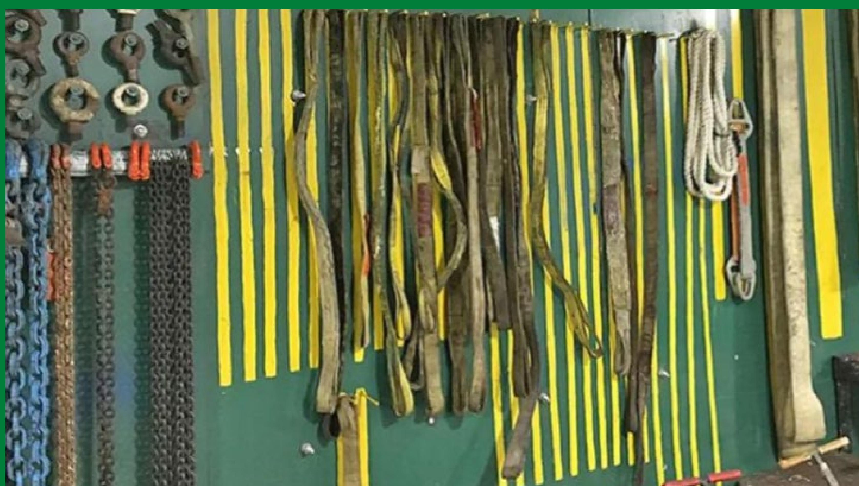
Keep slings clean and free of debris but do not use solvents or degreasers on nylon, polyester, and synthetic fiber, or fiber core wire rope slings.
