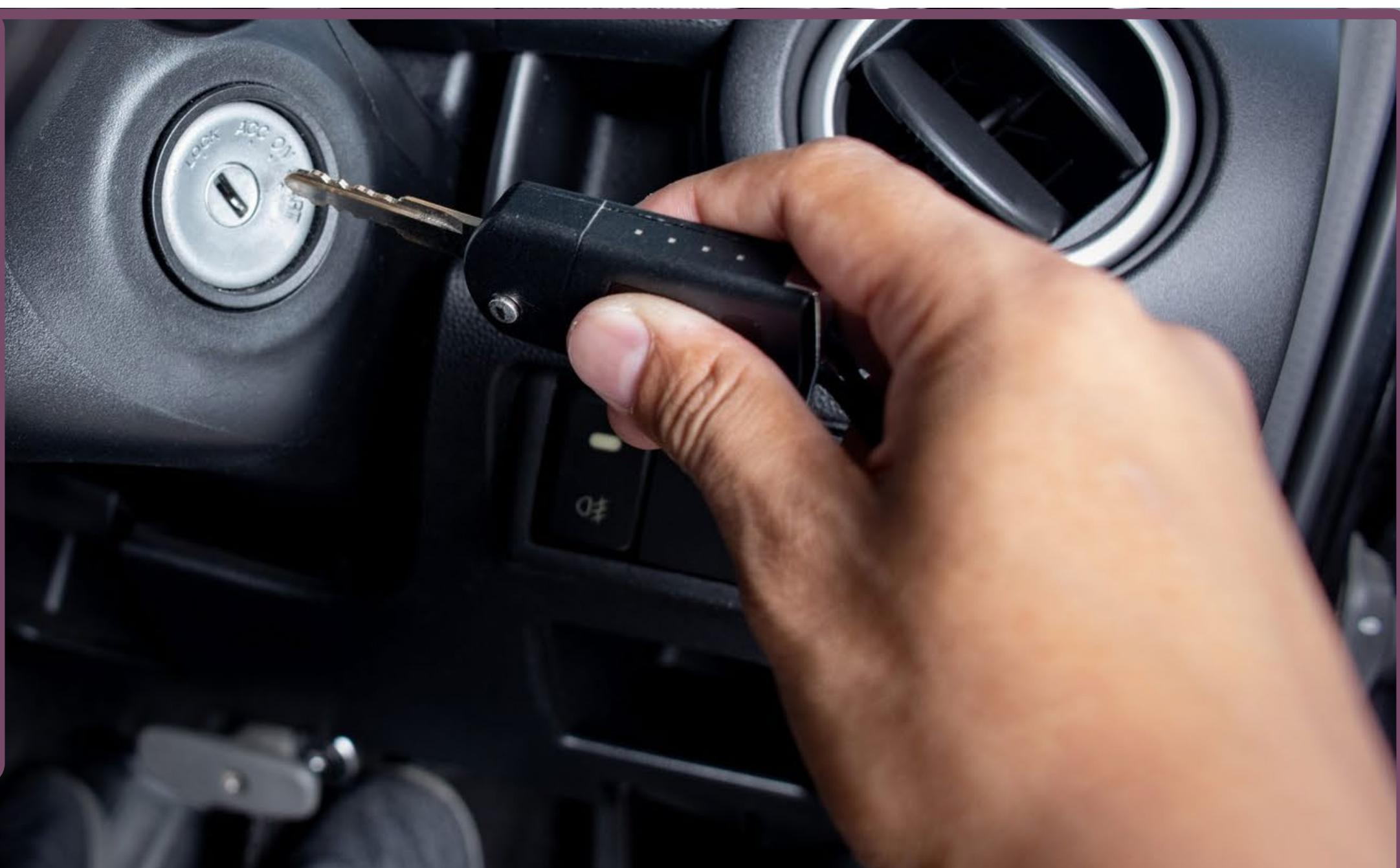
Every time locks are applied, they must be verified by a second mechanic (verifier), supervisor, or equipment operator. The lockout verifier is verifying the energy is isolated and that the lock has been applied.
