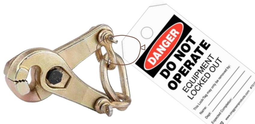
**3** If the Mobile Equipment does not have a night switch lock out point, then remove the key and lock it to the steering wheel with a scissor clamp, personal lock, and information tag.
