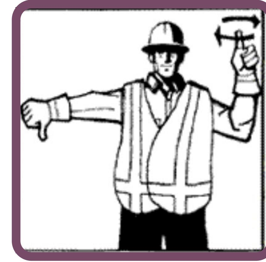
**Lower the boom and raise the load:** Arm extended, fingers close thumb pointing downward, other arm with forearm vertical, forefinger pointing upward and rotate hand in horizontal circles.
