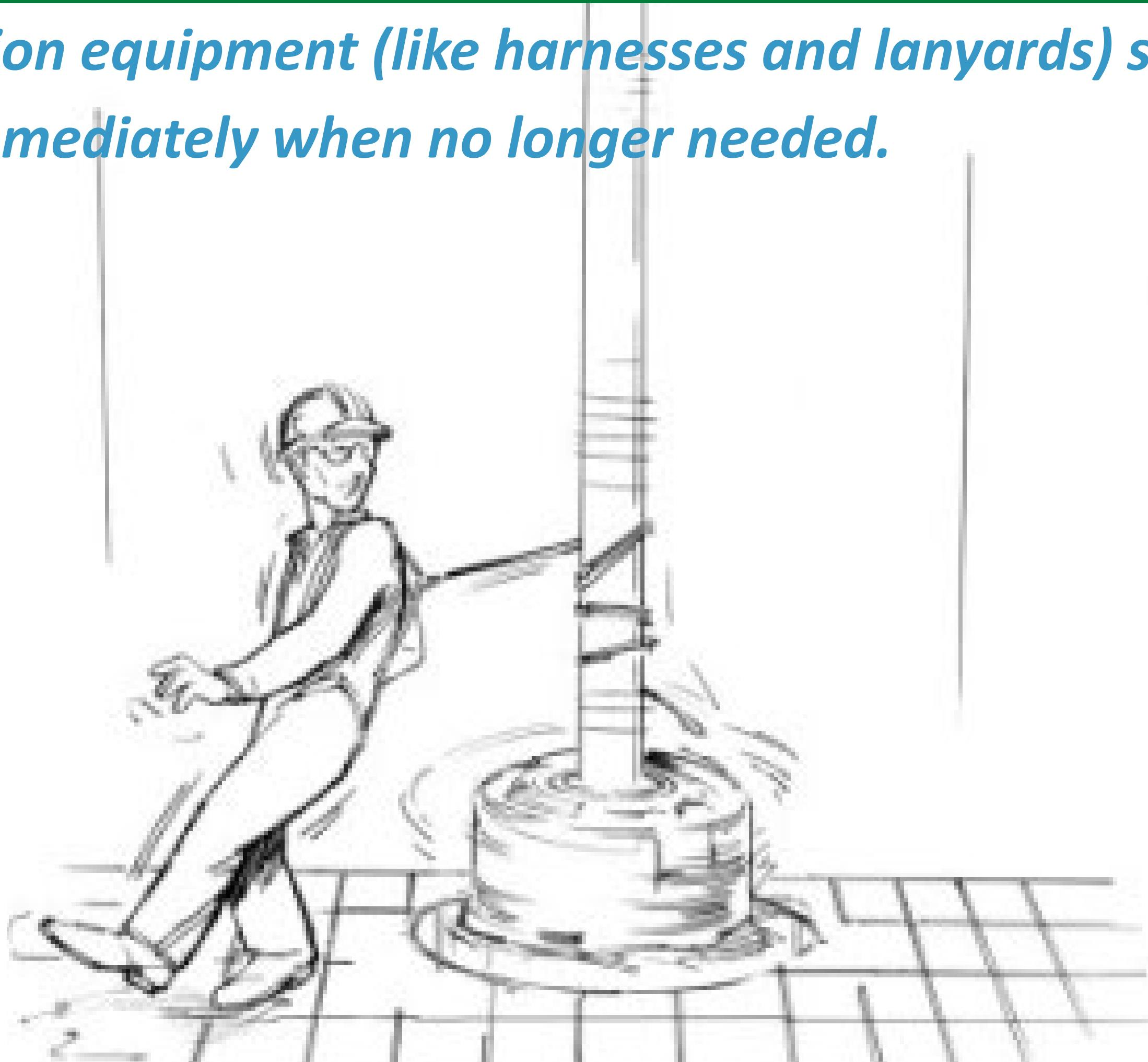
There have been multiple occurrences throughout manufacturing facilities where a lanyard has become caught or entangled in moving equipment, after the worker's task had been completed and the equipment should have already been removed.
