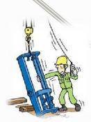
**Ensure that while** guiding a load with a tag line that your travel path is clear and safe before the load is suspended. DANGE
