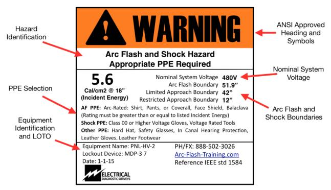
Above is an example of the labels you will find on MCC's, Disconnects etc. As you can see, we can learn a lot about the hazards associated with electrical equipment:
